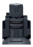
The Type 546 Ball Valve stem utilizes a predetermined break point opposite the media side of the stem seals. This break point is a groove with an inner diameter that is less than the stem seal grooves. This ensures that if there is a stem failure, the failure will occur at that point and media will not leak to the outside of the valve.
