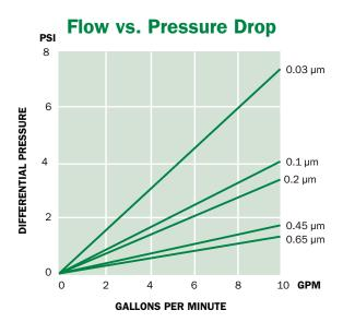
This chart represents the typical water flow per 10" cartridge length. Cartridges are tested in water at ambient temperature. Data may be extrapolated for multiple lengths, but as flow rate increases,  $\Delta P$  of the housing becomes more apparent.
