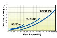
Above: Pressure drop is for filter housing and 20 micron filter cartridge in clean water.
