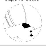
Detail of Protected seat & encapsulated body seal design. Isolates & protects both seats and seals from flow path. Helps to prevent cold flow.
